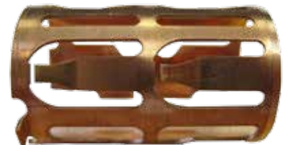
Beryllium-copper clamping sleeve (old)
